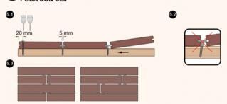
BOARDS MUST BE FIXED WITH CLIPS IN CORRESPONDENCE WITH EACH JOIST. EVERY BOARD END MUST BE FIXED WITH TWO CLIPS. IF NECESSARY, DOUBLE THE JOIST. EVERY END OF THE BOARDS MUST BE FIXED WITH TWO CLIPS
