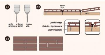
BOARDS MUST BE FIXED WITH CLIPS IN CORRESPONDENCE WITH EACH JOIST. EVERY BOARD END MUST BE FIXED WITH TWO CLIPS. IF NECESSARY, DOUBLE THE JOIST.
